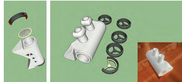
Figure 3. Computer draft and FDM printed model of nasal device
