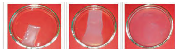
Figure 2. Disintegration behaviour of alg-gNCC film in contact with water (at 0, 2 min and 20 min from left to right).
